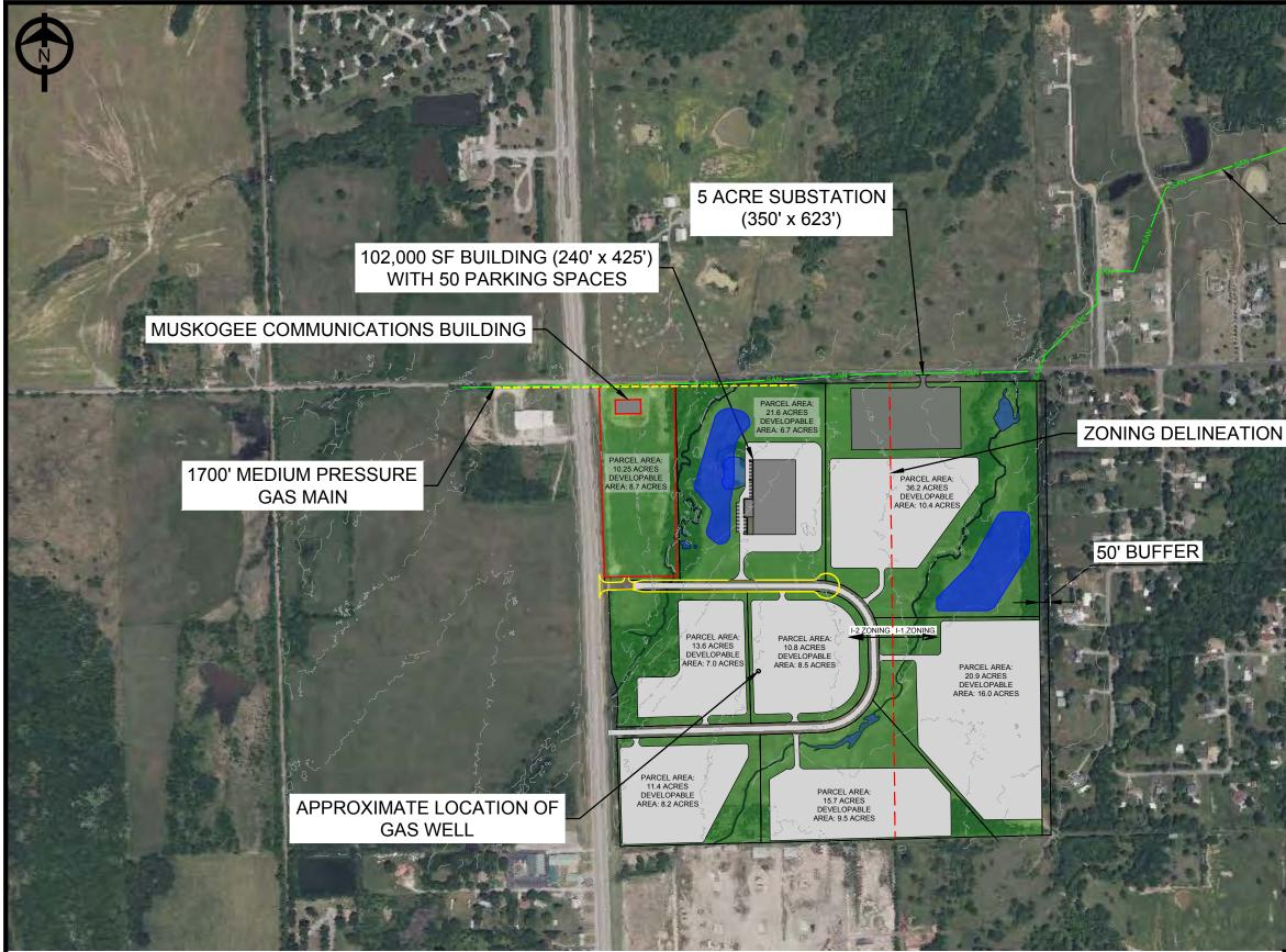
**NOTE:** ALL ACREAGES ARE APPROXIMATE. WILL NEED TO FINALIZE AREAS DURING DETAILED DESIGN. WILL NEED TO CONFIRM THAT 53RD STREET HAS AN ADEQUATE PAVEMENT SECTION FOR TRUCK TRAFFIC WITH HEAVY LOADS. 50' BUFFER APPLIED TO ALL DEVELOPMENTS IN CLOSE PROXIMITY TO STREAMS.
